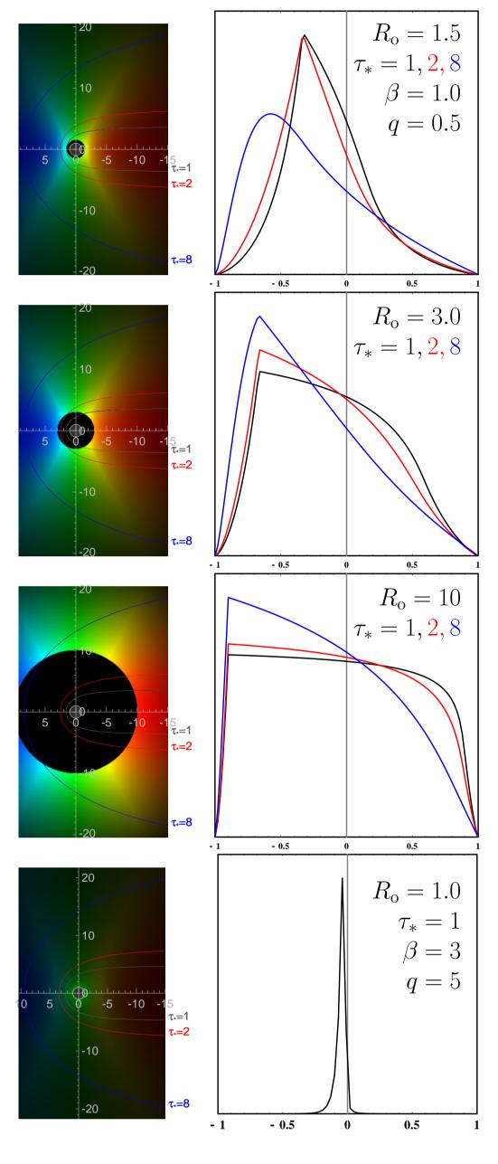
**Contours of optical depth** unity overlaying color velocity maps (far left) with corresponding line profiles (immediate left) for different values of  $\tau_*$ .
