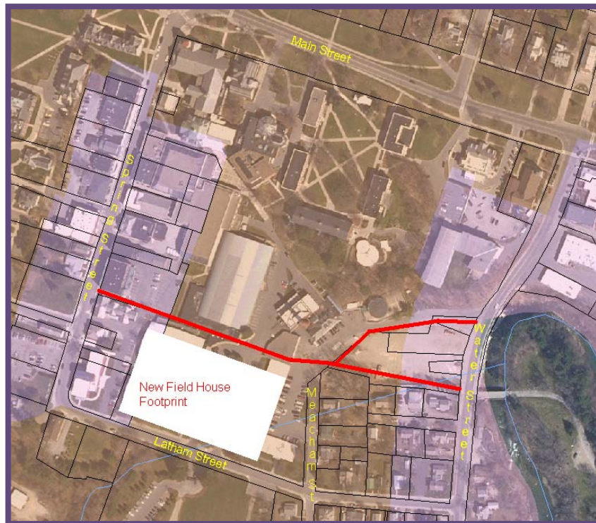
Figure 7 – Illustrates the rotated and enlarged design for the College field house, running parallel to Latham Street, and allowing room for the connection pathway.
