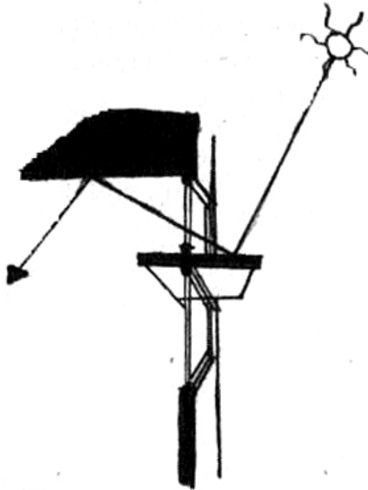
An example of a light shelf that indirectly bathes the interior in glare-free natural light while shading the view glass from direct glare.
