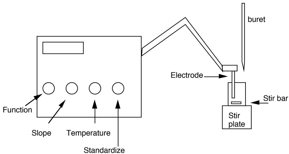
**Figure 1.** Set-up for titration using the Acumet pH meter.
