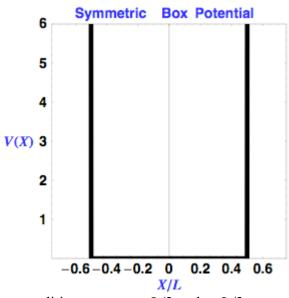
Notice that the boundary conditions are at x=-L/2 and x=L/2.
