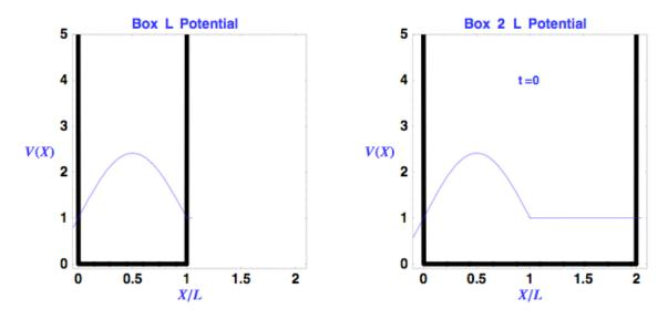
After the change, if we measure the energy the system would collapse into one of the new eigenstates. What is the probability of finding the state in the ground state, and first excited state of the new potential?
