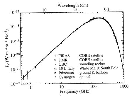
The figure shows that the background radiation follows the blackbody distribution. From the figure estimate the temperature of the background radiation of the Universe.
