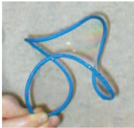
Figure 1: Soap films seek the least-area way to span a wire boundary, Photo by S. Devadoss.
