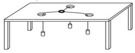
Theorem: A central, moveable point connected to a set of points via weights and strings will be at equilibrium if and only if it is also located at a mediancentre of the set of points.
