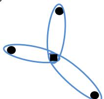
Theorem: A central, moveable point connected to a set of points via ideal rubber bands will come to rest at the mean location of the set of points.
