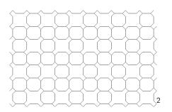
Note that the cornered tiles must alternate every row or column and cannot be "back-to-back"
