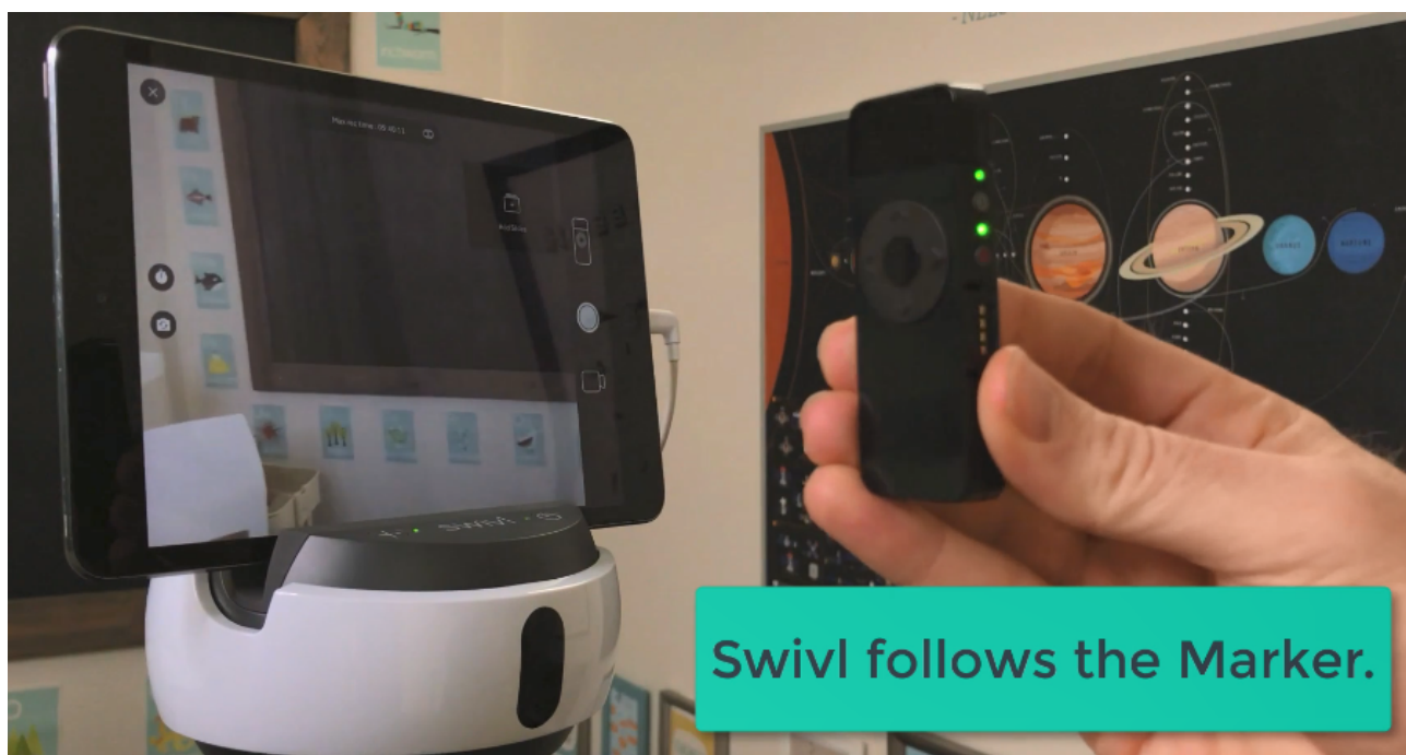
Figure 5. Swivl system for tracking lectures, image from their homepage ( https://www.swivl.com/how-to-use/ ). Note the instructor can see what is being recorded in the iPad screen, and the system follows the tracker in real-time.
