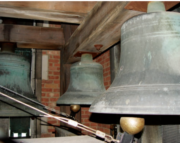
In performance, the inner wall of each of the tower's stationary bells is struck by a hammer connected by a long cable to its corresponding keyboard baton way below.
