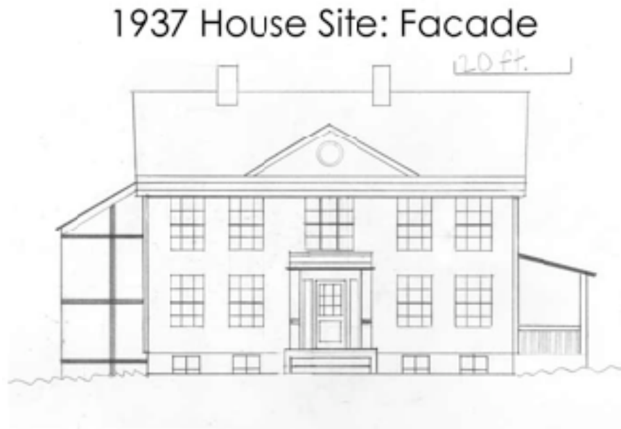
Figure 21: A potential elevation of Kellogg with its additions on the left and a small porch on the right
