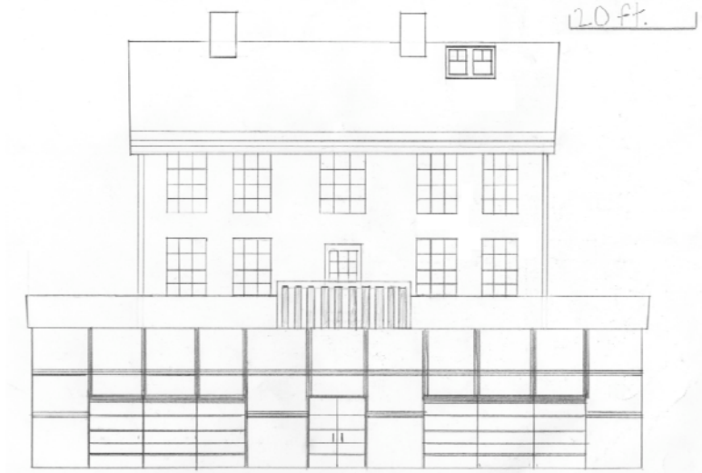
Figure 24: Rear elevation of Kellogg on the Seeley Site including glass addition with sliding garage doors opening up to garden and small porch overlooking garden on roof of addition.
