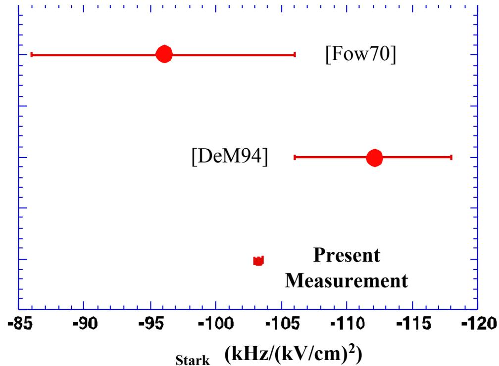
**Our Measurement:**  $\text{Stark} = 103.23(39) \text{ kHz}/(\text{kV}/\text{cm})^2$
