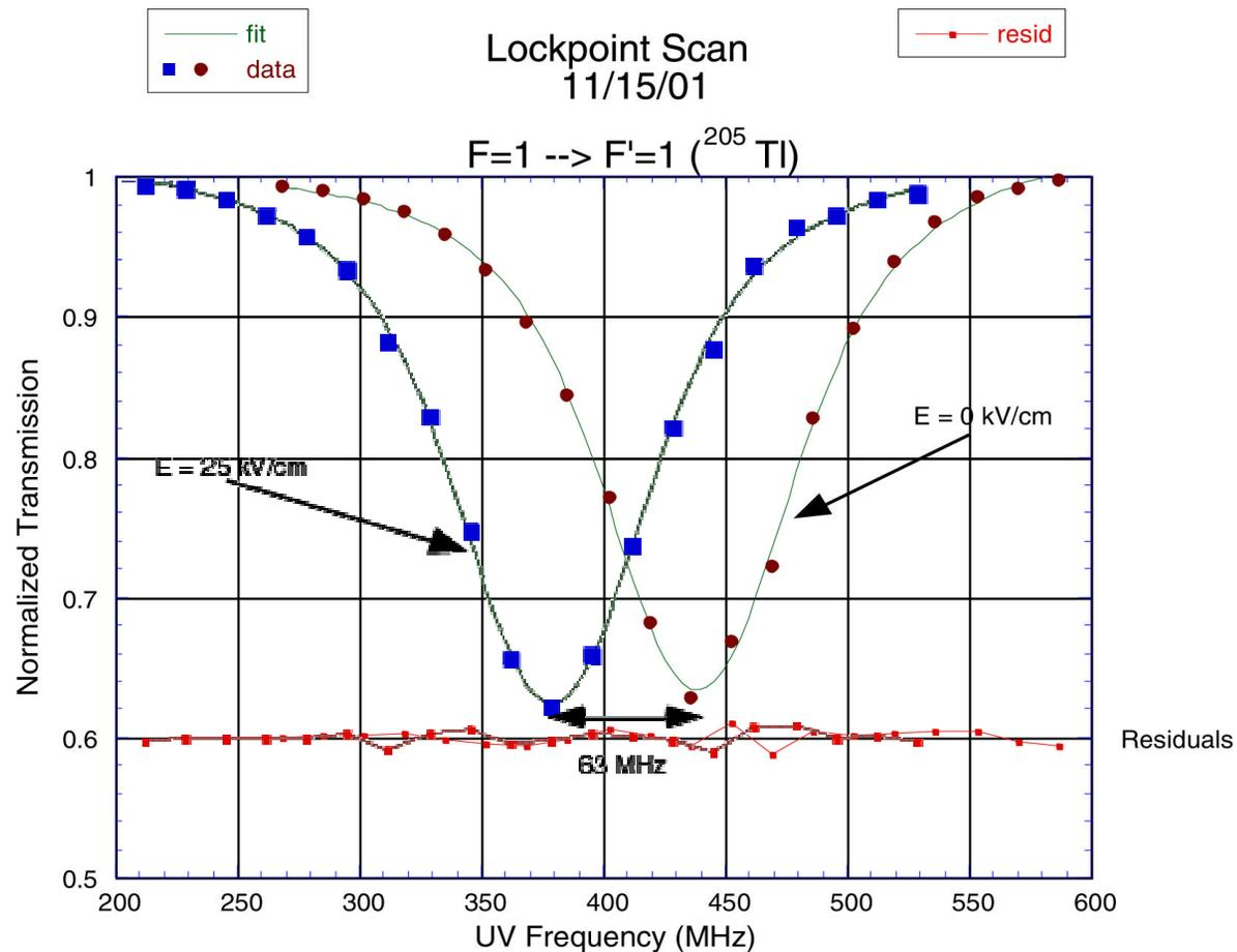
$$\text{Stark} = \frac{63 \text{ MHz}}{(25 \text{ kV/cm})^2}$$
