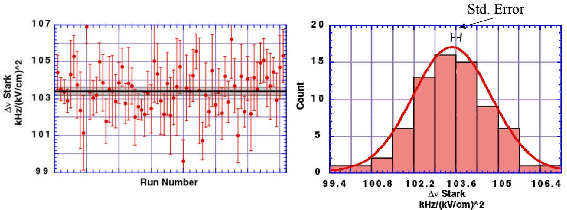
Final Statistical Error:  $0.20 \text{ kHz}/(\text{kV}/\text{cm})^2$  (0.19%)
