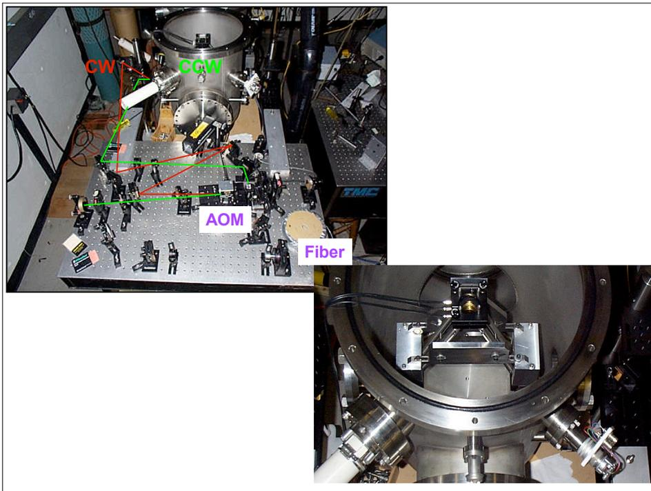
**Dual directional ring cavity transmission
